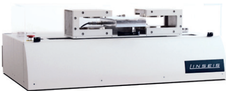
TFA with permanent magnet (up to 0.5 Tesla)
