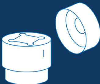
Sample holder square samples 3x3 mm / 10x10 mm / 20x20 mm
