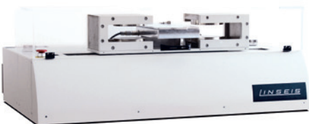
TFA with permanent magnet (up to 0.5 Tesla)
