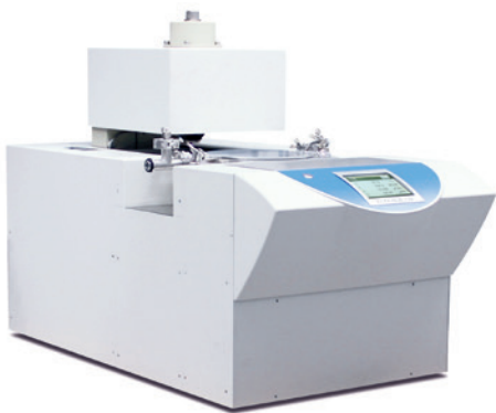
TFA with moveable electromagnet (up to 1 Tesla)
