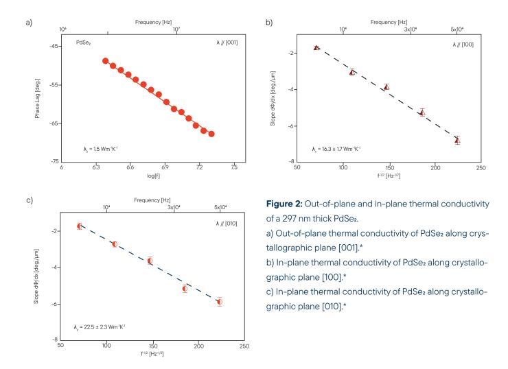
The **TF-LFA** offers the possibility to measure the thermal conductivity of such a 2D material not only in both major directions, in- and out-of-plane, (see Fig. 2 b & 2 c) even over the axis of rotation of the surface in two different crystallographic planes.
