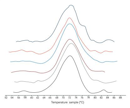
In biochemical, biophysical or pharmaceutical research, proteins are an important subject in the development of new drugs or treatments. The stability parameters of these proteins are necessary for all these developments, so it is essential to know, for example, the denaturation temperature of the proteins as well as the energy required for denaturation (denaturation enthalpy temperature). required.
