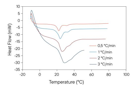
A 524 mg PTFE cylinder was placed in the measurement cell while the reference cell remained empty. The Ultimate Micro Calorimeter was programmed to perform several heating ramps between -10°C and 80°C, at scanning speeds of between 0.5 and 3°C/minute. The thermograms obtained are shown opposite. At all the speeds tested, the two Teflon phase transitions were observed. The separation of the two transitions is all the more marked on the thermograms when the scanning speed is low.
