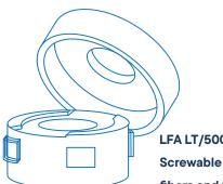
LFA LT/500/100 Screwable sample holder for fibers and foils
