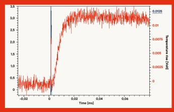
Measurement with conventional light guiding system\* \*Multiple light guides are available for samples from 6 to 25.4 mm
