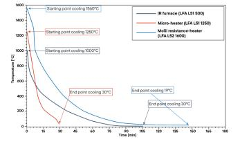
Cooling comparison of IR furnace, micro-heater, and MoSi resistance-heater clearly demonstrates the advantage of short cool-down times. This allows multiple measurements in quick succession and improves sample throughput. The IR furnace cools from 1000°C to 30°C in 105 minutes, while the microheater takes only ~26.5 minutes. Even when cooling from 1250°C, it stays below 30 minutes. The MoSi-heater, used for comparison, cools from 1560°C to 19°C in approximately 147 minutes.
