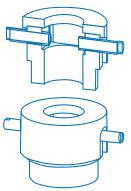
LFA LT/500/100 Sample holder for lamellas Ø 10 mm x 10 mm
