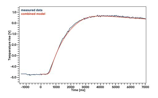
Temperature rise of the PMMA sample (length 1.01 mm, half time rise 1218.75 ms). The combined model illustrates a perfect fit to the data points
