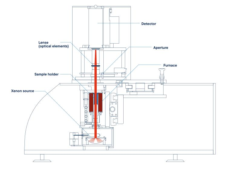
The Linseis **LFA L51 1250** features a vertical configuration with the detector positioned above the sample and the Light Flash source below. This design facilitates straightforward handling and optimal measurement outcomes. The five micro-heaters heat ultra-fast, which minimizes the total measuring time and increases the throughput.
