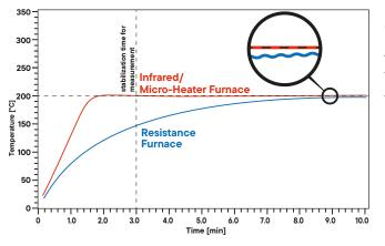
Comparison of time to reach the temperature stability. A high speed IR-micro-heater furnace reaches the set temperature much faster and delivers a superior isothermal temperature stability.
