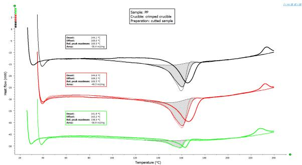
reproducibility. The crimped crucible is working as a susceptor here, causing a homogenous heat around the sample. Furthermore, the good sample contact and lowered heat capacity have a positive effect on the sample and the shape of the peak.
