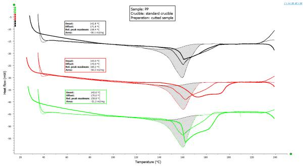
can be improved a lot. Anyway, the first run of these samples is inconsistent due to different melting behaviour of the different shaped samples.
