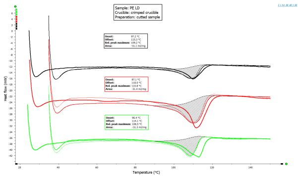
reproducibility. The crimped crucible is working as a susceptor here, causing a homogenous heat around the sample. Furthermore, the good sample contact and lowered heat capacity have a positive effect on the sample and the shape of the peak.
