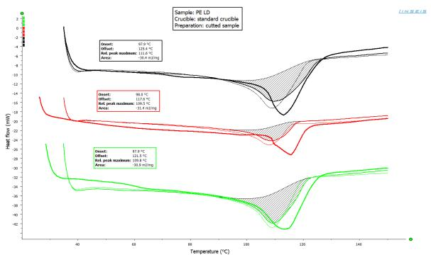
Evaluated is the second peak and it makes clear even with a pity effort on sample preparation the results can be improved a lot. Anyway, the first run of these samples is inconsistent due to different melting behaviour of the different shaped samples.
