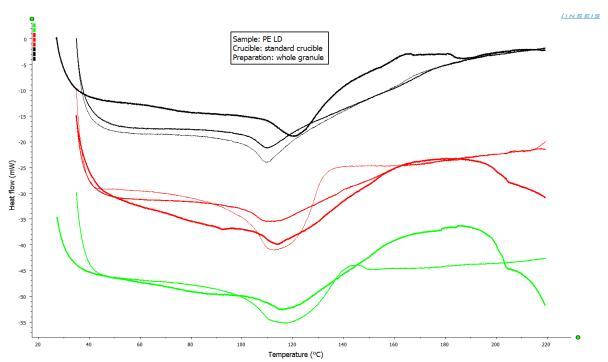
As shown in the diagram, it's almost not possible to receive any reproducible values from these tests. During the first cycle the sample is melting and receive a better contact to the crucible whats visible on the measurement signal. But it last three runs until the sample is complete melted. Furthermore the sample does not melt into the crucible but moves out of the crucible which makes it impossible to receive a reproducible contact.
