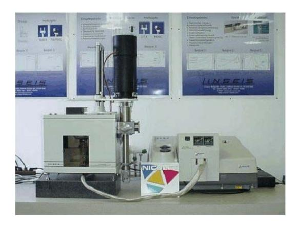
In cooperation with the company Nicolet, the company Linseis Messgeräte GmbH has realized a coupling of thermobalance with DTA or HDSC - measuring system and an infrared spectrometer of the type NEXUS and now currently in the scope of delivery.
