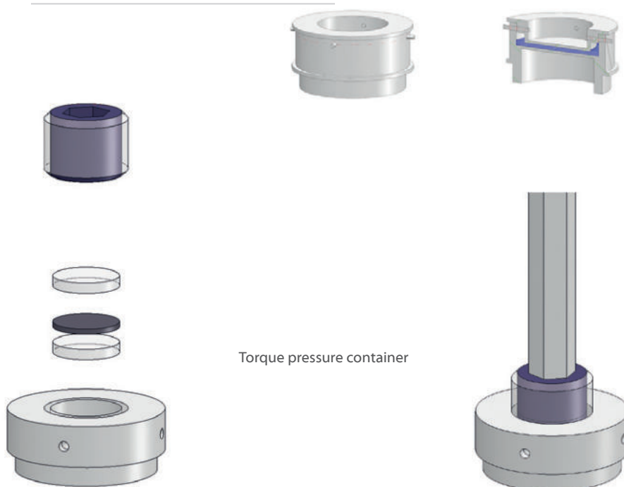
Sample holder for liquids and pastes
