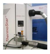
Now on top of information about the weight change of temperature, enthalpies, specific heats and the general behaviour under temperature changes, a full evolved gas analysis can be performed. The knowledge of these gases, which were burned off in the balance, leads to the understanding of which products have been burned off.
