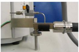
Linseis Instruments has developed in cooperation with JASCO Corporation a coupling between a thermal balance L81/1550 and a JASCO FTIR Spectrometer series 460.
